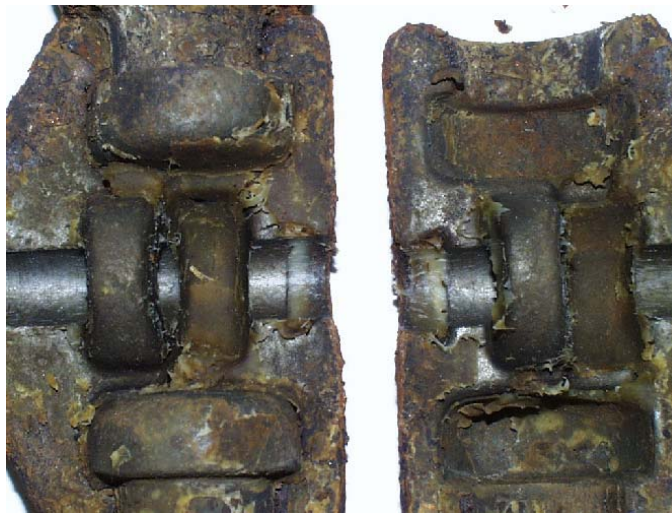
Figure 2: Interior Surfaces of Link Containing E-2000 After 150 Cycles Of Cyclic Test Exposure
