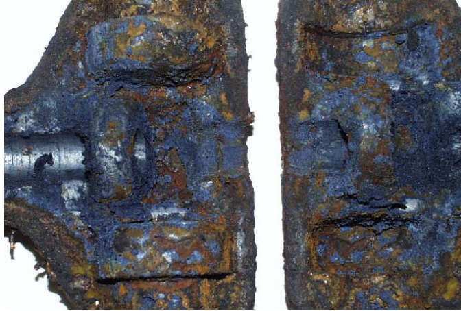
Figure 1: Internal Surfaces of Link Containing E-1000 After 150 Cycles Of Cyclic Test Exposure
