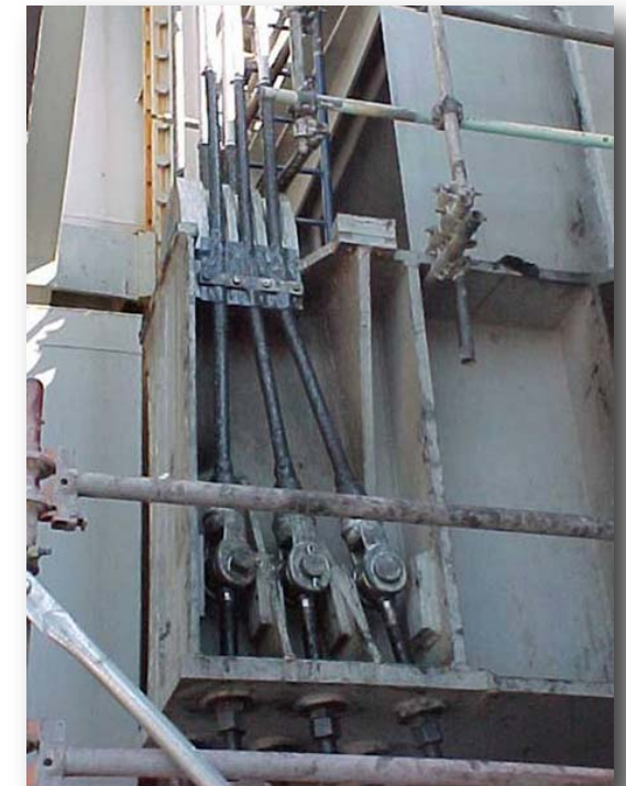
Typical Corrosion on Deck Edge Elevator Cables
