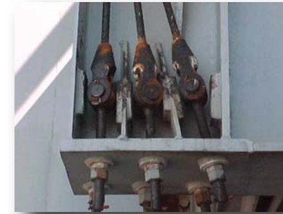
Typical Corrosion on Deck Edge Elevator Cables
